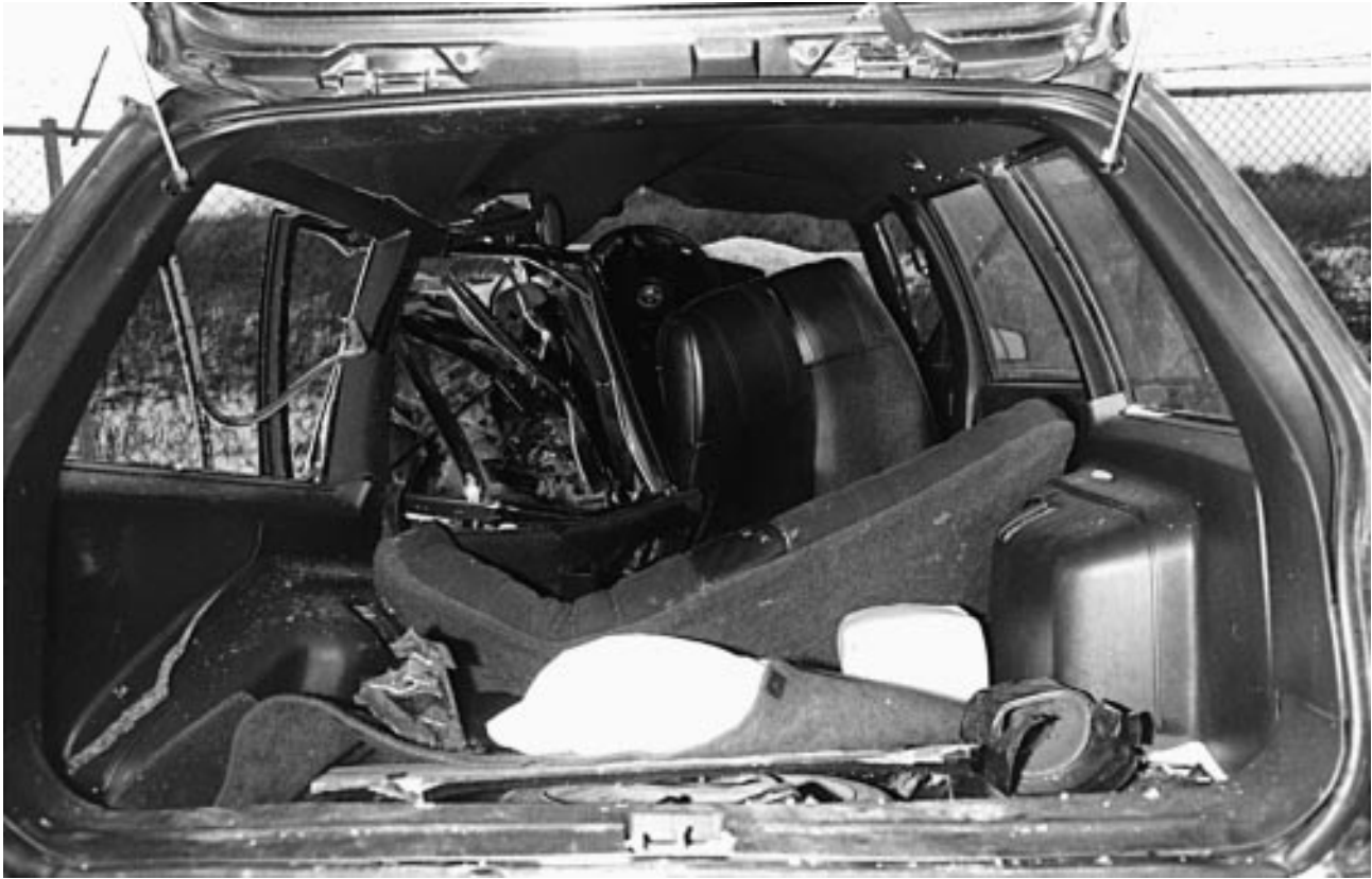
FIG. 5—Thirty-five-year-old restrained male driver: isthmic rupture. Oblique near-side impact with car ( EBS = 69 \text{ km/h} ; 43 \text{ mph} ). Massive intrusion at driver's door. Other major injuries cardiac laceration, bilateral rib fractures with left diaphragmatic tear, splenic and mesenteric lacerations, fracture of T_5 - T_6 , tear of the upper abdominal aorta.
