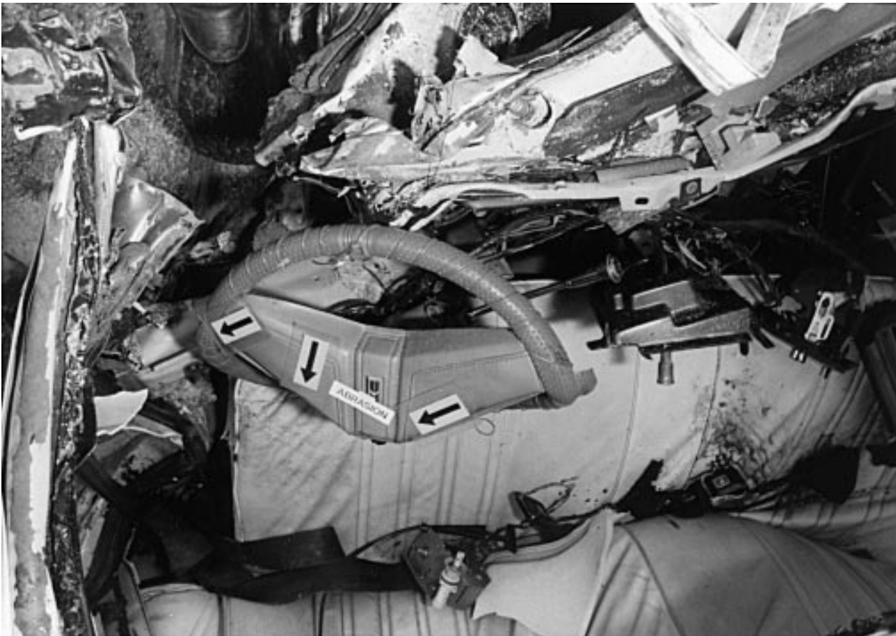
FIG. 2—Eighteen-year-old restrained male driver suffered complete aortic transection at isthmus following collision with heavy truck. Severe passenger compartment intrusion. Chest contact (“abrasion”) with steering wheel that shows major deformation and rotation upward. Fracture of sternum. Ribs intact. Hepatic, splenic and jejunal lacerations.
